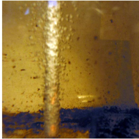
Gas bubbles generated by ultrasound on a wire surface
