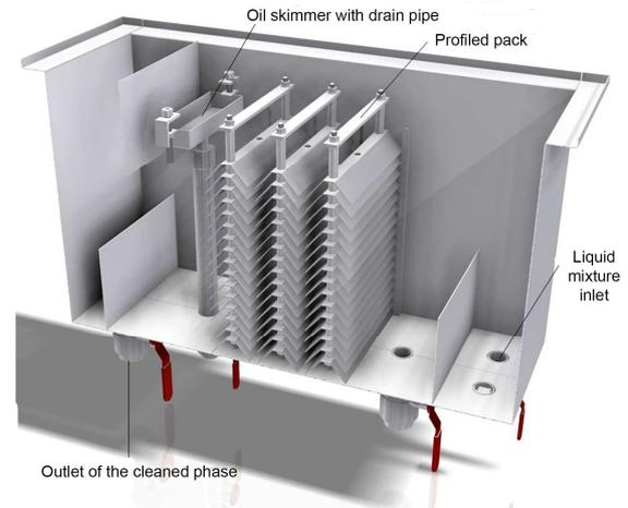
**Plate phase separator for separating the oil phase**
